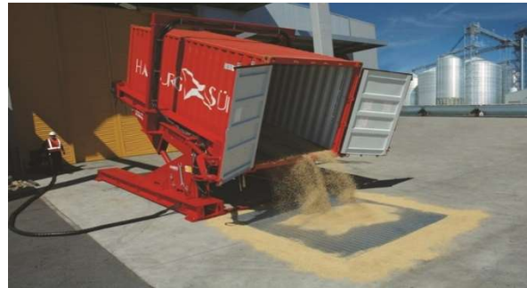
Unloading by Container Tilter in procuring Silos
