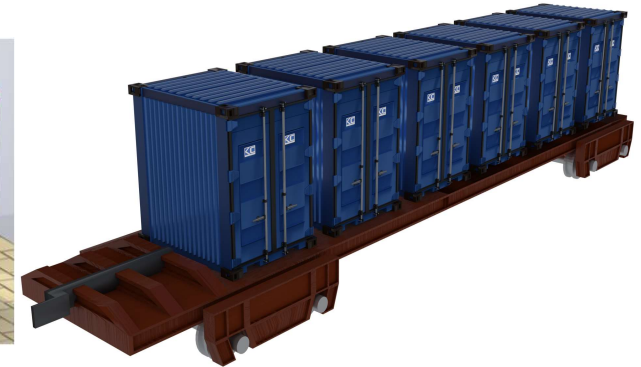
6 Cuboid on one wagon i.e. 48 bike /wagon and 2160 bikes per rake For Longer Journey
