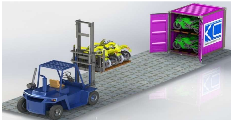
Two Bike Stand in a Cuboid i.e. 8 Bike per container
