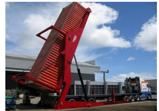
Unloading at Consuming SILO by Tilter
